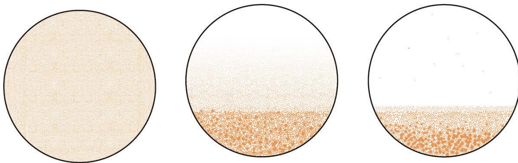
Figure 28. Three transport regimes in a pipe; non-settling or homogeneous (left), partially stratified or heterogeneous (middle), and fully stratified (right).
