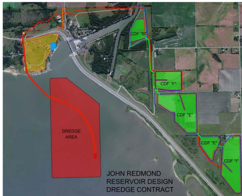
Figure 24. The dredge area of John Redmond Reservoir on the Neosho River in eastern Kansas was close to the dam and disposal areas. The red line on the drawing is the dredge discharge pipeline (figure courtesy of Jim Ho, GLDD AutoCAD Department).
